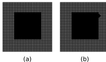
Figure 5: (a)the input pattern of good part which is rotated by  $0^\circ$ . (b) the input pattern of bad part which is rotated by  $0^\circ$ . the area of deformation occupies about 0.7% of the area of good part.
