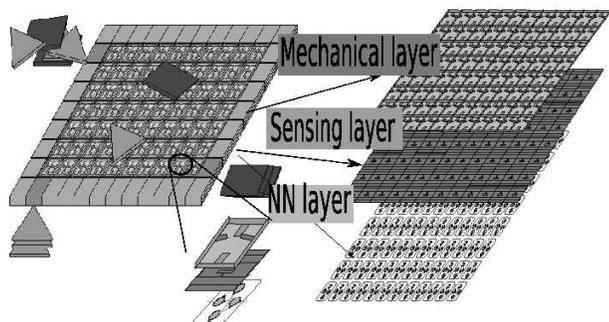
Figure 1: Our goal. This system composes three layers, which are actuator, sensor and NN.
